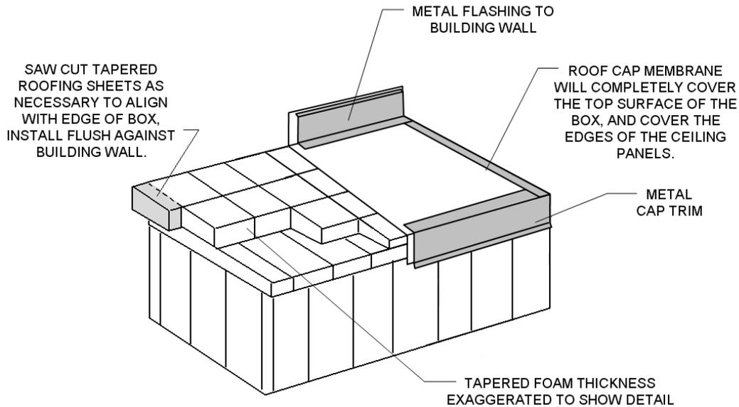
The tapered roof system consists of tapered foam sheets, rolled polyethylene roof cap membrane, flashing, roof cap trim, and fasteners. Installation is identical to standard membrane roofs with the exception of adding the sloped foam sheets. In applications with very large roofs, multiple layers of sloped foam may be required.
